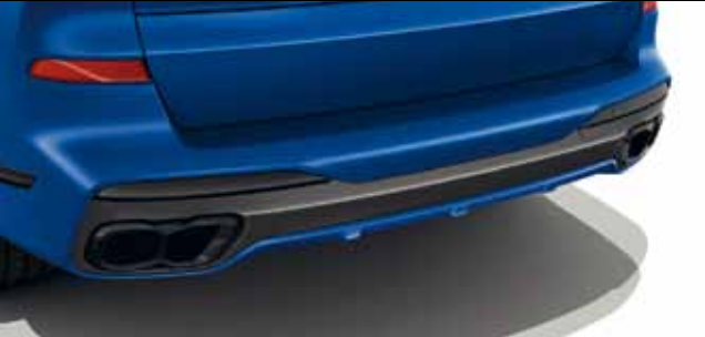
The M sport exhaust system delivers a sound that can be adjusted to an even more intense engine sound with the driving dynamics buttons in the SPORT and SPORT+ programmes, while the comfort-oriented programme prioritises more discreet engine acoustics.
