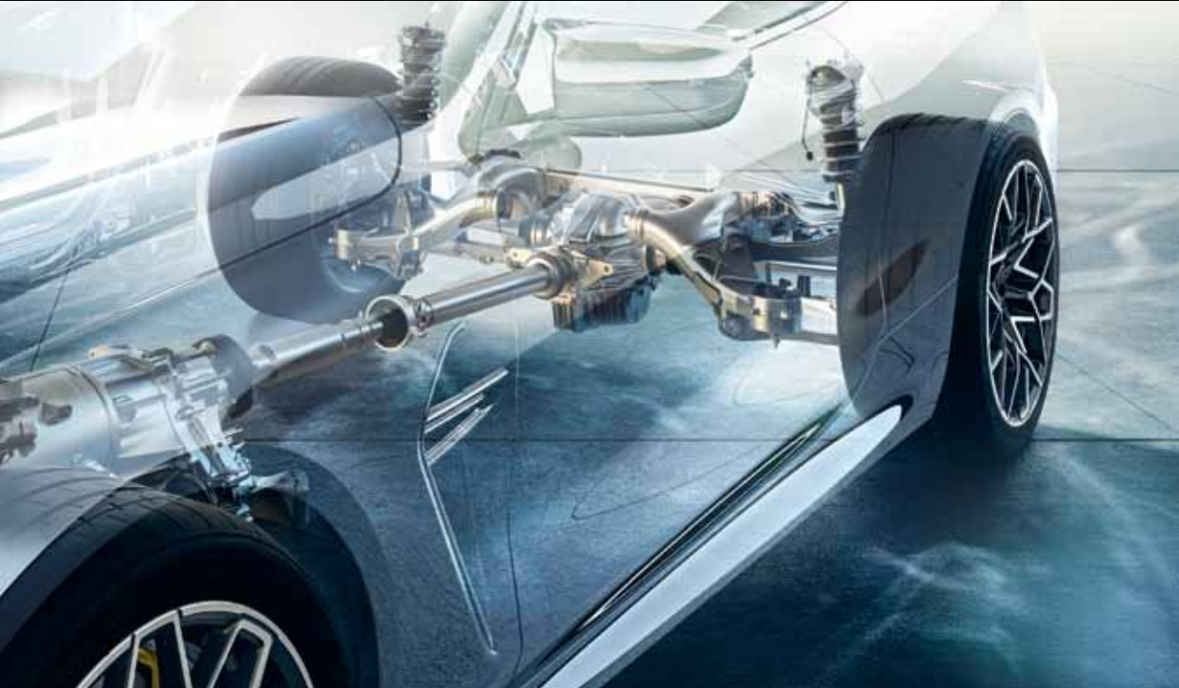
□ The Adaptive M suspension Professional 1 guarantees optimum driving stability and dynamics via the active roll stabilisation.
