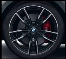
19" M light alloy wheels Double-spoke style 792 M Bicolour Jet Black with performance tyres and mixed tyres, gloss-lathed, front 8J x 19 with 225/40 R19 tyres, rear  $8.5J \times 19$  with 255/35 R19 tyres.
