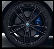
19" M light alloy wheels Double-spoke style 791 M Jet Black uni with performance tyres and mixed tyres, wheel size front 8J  $\times$  19 with 225/40 R19 tyres, wheel size rear 8.5J  $\times$  19 with 255/35 R19 tyres.
