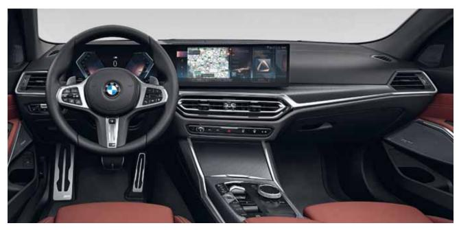
BMW Live Cockpit Professional with its large curved display expands BMW Live Cockpit Plus with a full-colour head-up display. This projects driving information such as speed or navigation instructions directly into the field of vision — for a better overview and more safety.
