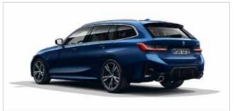
18" M light alloy wheels Doublespoke style 848 M Bicolour Jet Black with mixed tyres, gloss-lathed, wheel size front 7.5J x 18 with 225/45 R18 tyres, wheel size rear 8.5J x 18 with 255/40 R18 tyres.
