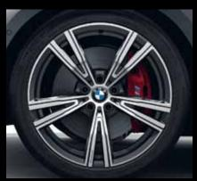
19" BMW Individual light alloy wheels Double-spoke style 793 I Bicolour Orbit Grey with mixed tyres and run-flat tyres, gloss-lathed, wheel size front 8J x 19 with 225/40 R19 tyres, wheel size rear  $8.5J \times 19$  with 255/35 R19 tyres.
