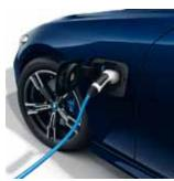
With the standard charging cable (mode 2) for domestic socket outlets, you can conveniently charge your BMW's high-voltage battery at domestic sockets.
