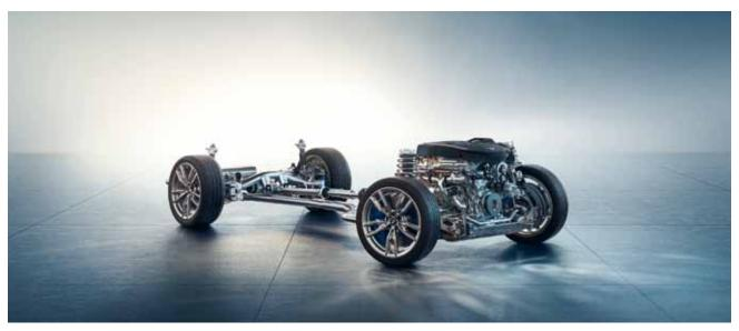
M Sport suspension¹ – which includes a suspension which is lowered by 10 millimetres – is characterised by more athletic suspension settings with tighter damper settings. It also features a moderately higher spring constant and harder stabilisers. Combined together, they result in an even more direct suspension design, which enables a distinctly sporty driving style.
