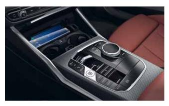
The wireless charging tray conveniently charges your smartphone without cables at up to 15 W of power. Integrated cooling protects against overheating.
