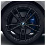
19" M light alloy wheels Doublespoke style 791 M Jet Black uni with performance tyres and mixed tyres, wheel size front 8J x 19 with 225/40 R19 tyres, wheel size rear  $8.5J \times 19$ with 255/35 R19 tyres.1
