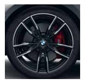
19" M light alloy wheels Doublespoke style 792 M Bicolour Jet Black with mixed tyres and runflat tyres, gloss-lathed, front  $8J \times 19$  with  $225/40 \text{ R}19 \text{ tyres, rear } 8.5 \text{J} \times 19$ with 255/35 R19 tyres.4
