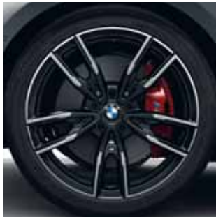
19" M light alloy wheels Double-spoke style 792 M Bicolour Jet Black with mixed tyres and runflat tyres, gloss-lathed, front 8J x 19 with 225/40 R19 tyres, rear 8.5J x 19 with 255/35 R19 tyres. 2
