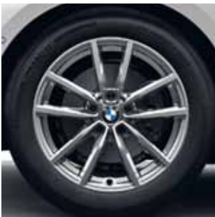
17" light alloy wheels V-spoke style 778 Reflex Silver, wheel size 7.5J x 17 with 225/50 R17 tyres. 4
