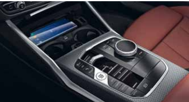
The wireless charging tray conveniently charges your smartphone without cables at up to 15W of power. Integrated cooling protects against overheating.
