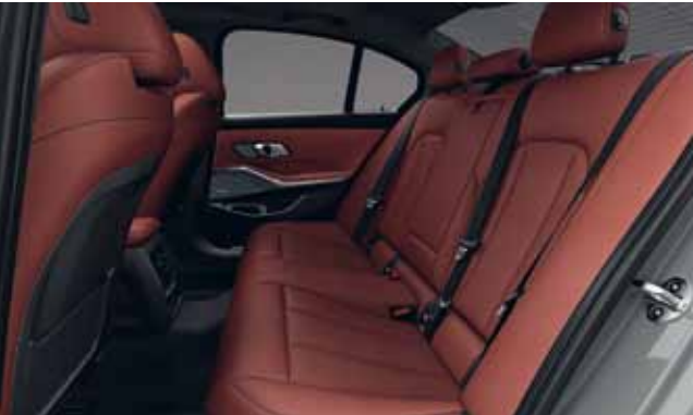
Folding rear head restraints for the three rear seats improve the view through the rear window.
