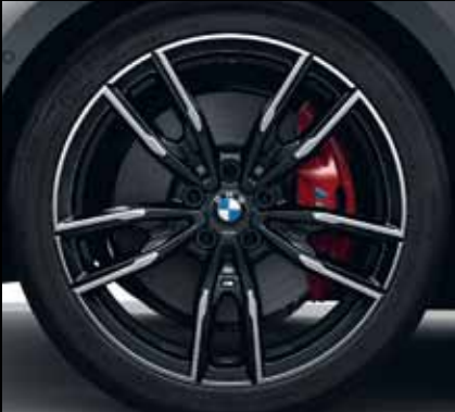
19" M light alloy wheels Double-spoke style 792 M Bicolour Jet Black with mixed tyres and runflat tyres, gloss-lathed, front 8J x 19 with 225/40 R19 tyres, rear 8.5J x 19 with 255/35 R19 tyres.
