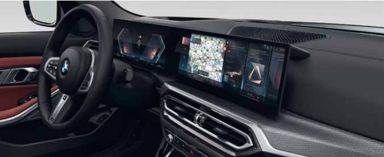
BMW Live Cockpit Professional with its large curved display expands BMW Live Cockpit Plus with a full-colour head-up display. This projects driving information such as speed or navigation instructions directly into the field of vision – for a better overview and more safety.
